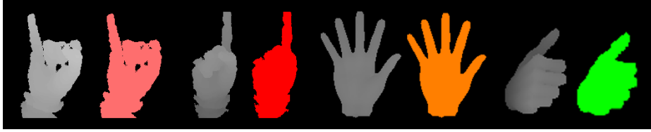
Fig. 2. SCT training images: The first four images are real depth images and their labels, and the rest of the images are synthetic depth images and their labels.
