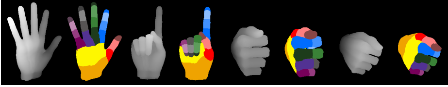
Fig. 3. Four examples of synthetic depth images and the corresponding ground truth labels that are used to train the pose estimation RDFs.
